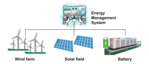
The EMS provides an integrated operation and revenue maximization system to renewable energy generation facility operators, by providing energy balancing and scheduling between various forms of renewable energy (wind, solar, etc.), conventional generation (thermal, hydro, etc.), energy storage systems (batteries, pumped hydro, and/or flywheels), and dispatch instructions from the market operator. Useful features include:
